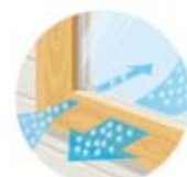
Water is repelled but micro porosity allows moisture to escape
